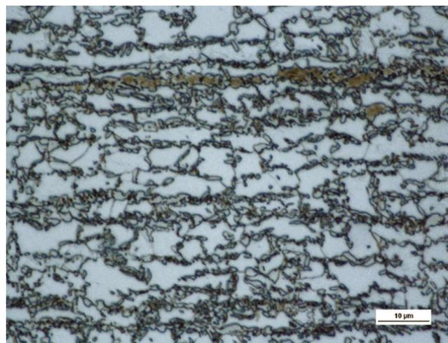
**Fig. 1.** TRIP steel microrstructure, LOM, Nital etched
