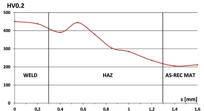
**Fig. 5.** Microhardness profile of fusion zone, TRIP steel
