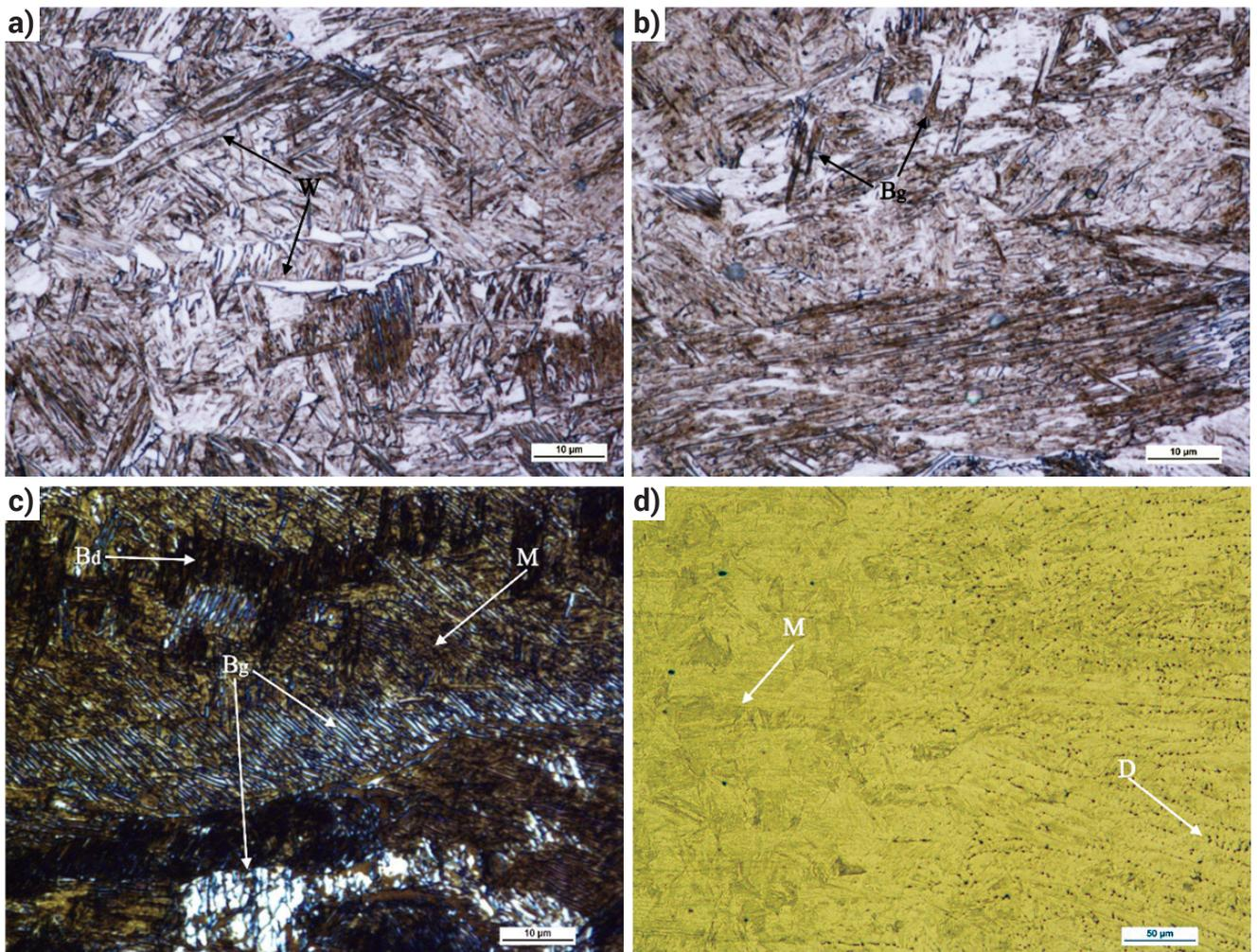
**Fig. 3.** TRIP steel microstructure, LOM: a) HAZ, Nital etched, b) Fusion zone, Nital etched, c) Fusion zone, Nital + Klemm reagent etched, d) Fusion zone and HAZ, Pikral etched
