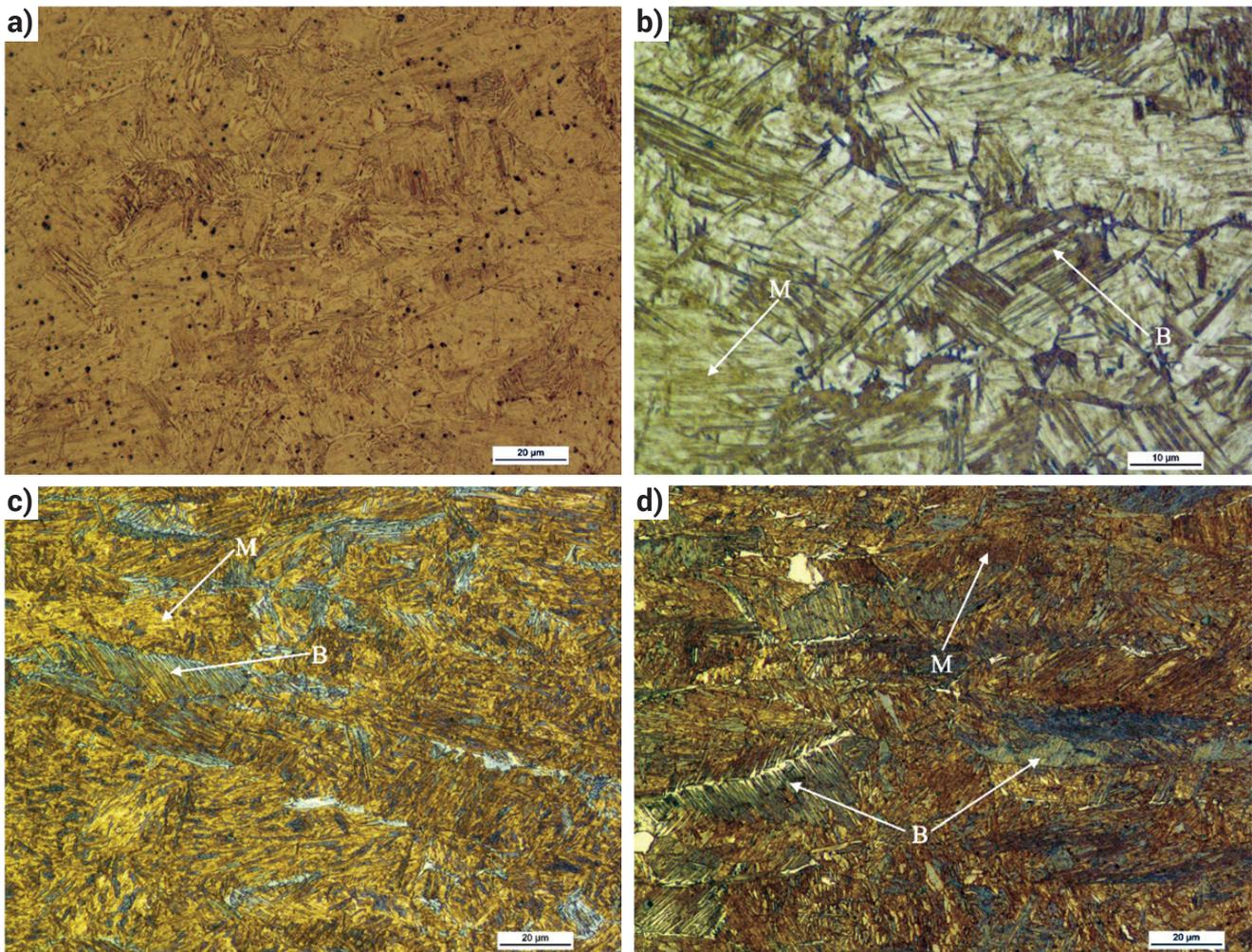
**Fig. 4.** Fusion zone microstructure, TRIP steel, LOM: a) Pikral etched, b) Pikral + LePera reagent etched, c) Pikral + LePera reagent etched, d) Pikral + sodium metabisulfite etched
