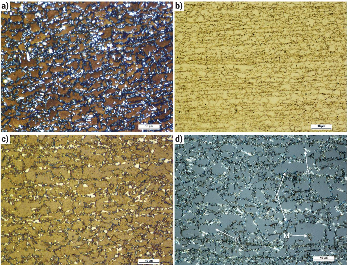
**Fig. 2.** TRIP steel microstructure, LOM: a) Nital + Klemm reagent etched, b) Pikral etched, c) Pikral + LePera reagent etchant etched, d) Pikral + sodium metabisulfite etched
