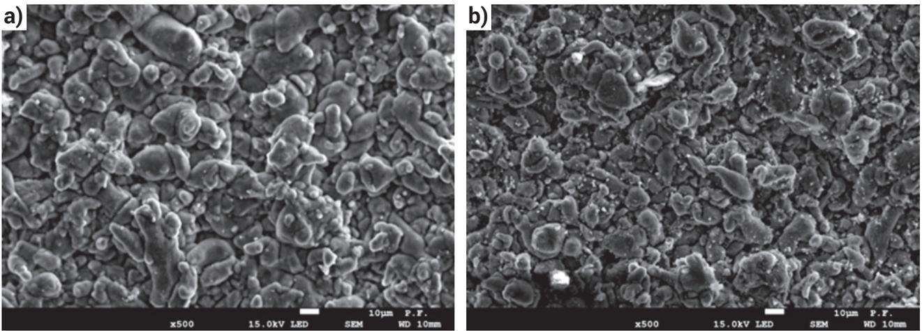
Fig. 3. Surface of aluminum coating sprayed with cold gas (500x magnification): a) on a 4330 steel substrate, b) on an Al 7075 alloy substrate
