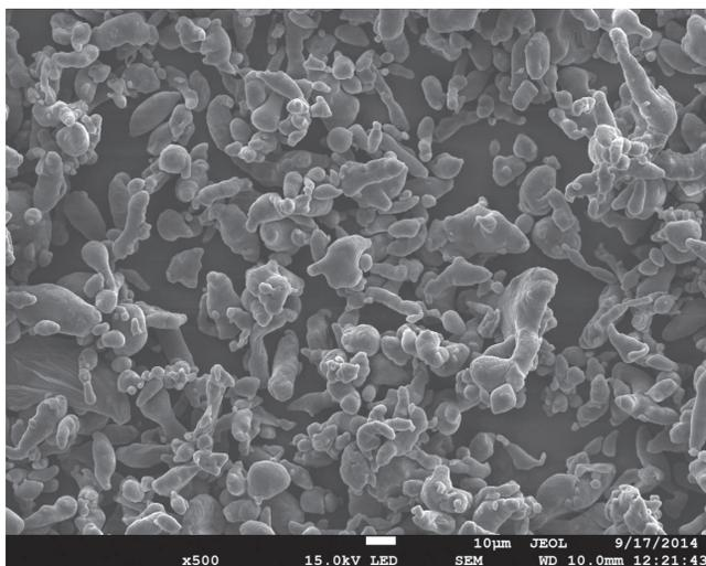
Fig. 1. Morphology of Al (500x magnification) powder grains
