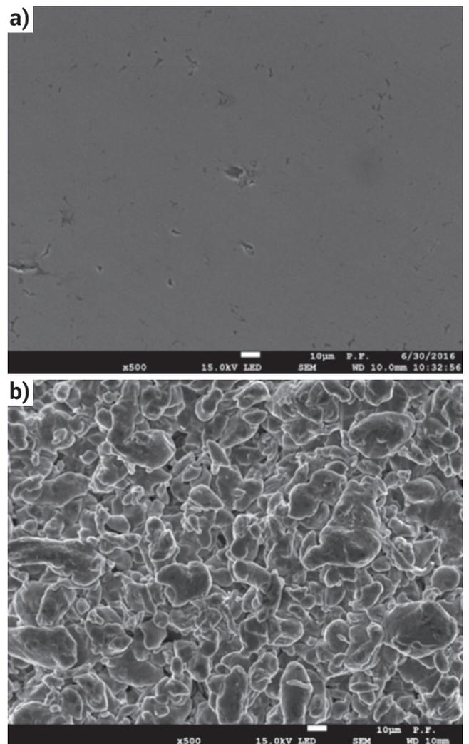
Fig. 2. Surface of samples used for testing (500x magnification): a) 4330 steel substrate, b) 7075 aluminum substrate
