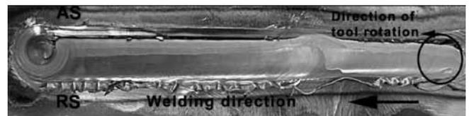
**Fig. 3.** Overall view on the surface of welded joint, 400 RPM 200 mm/min
