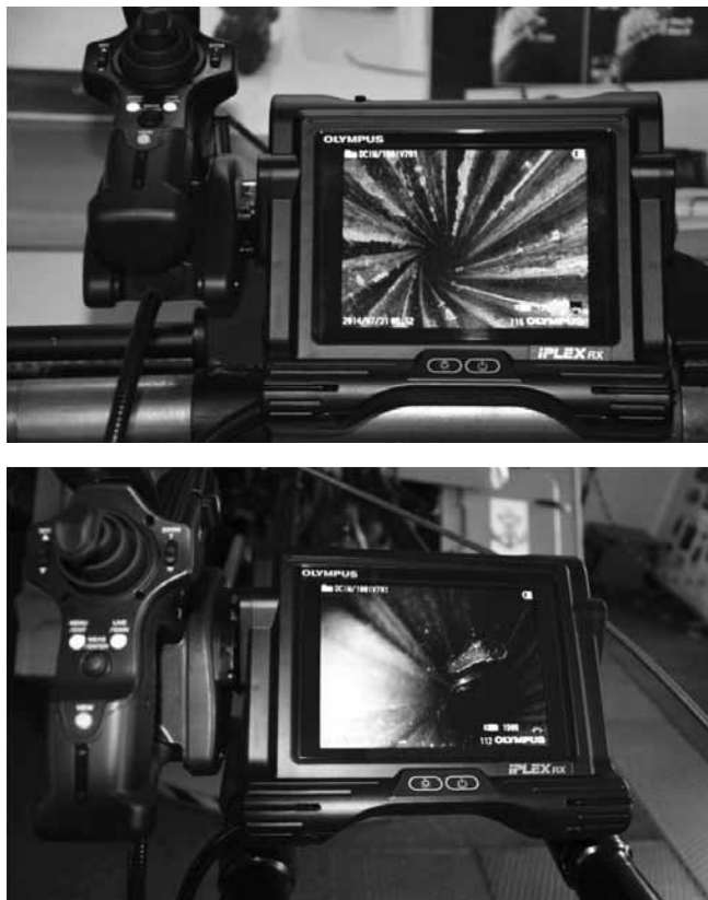
Rys. 3. Wideoskop iPLEX RX podczas badań luf armat morskich w PBRiA Fig. 3. iPLEX RX during the testing of marine cannon barrels in PBRiA
