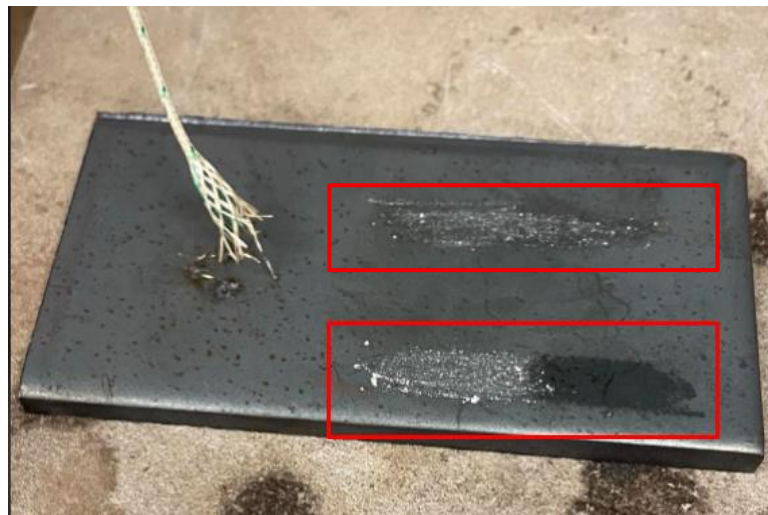
Fig. 6. Specimen during temperature indicator pens investigation
