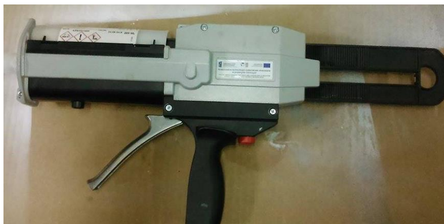
Fig. 3. Device for applying adhesive to the surfaces of araldite 2000 sheets
