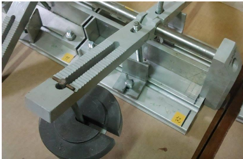
Fig. 2. Picture of the bonding device with the bonded sample attached
