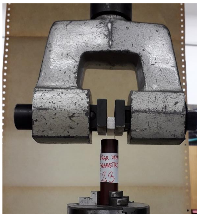
Fig. 5. Sample clamping on tensile strength measuring machine
