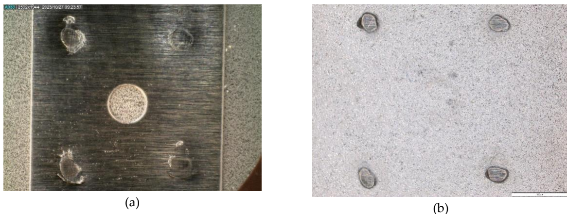
Fig. 7. Macro images of welds before (a) and after (b) tensile strength tests
