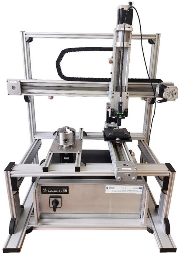
Fig. 2. The stationary automatic stand for non-destructive eddy current testing - AutoWIR-S1
