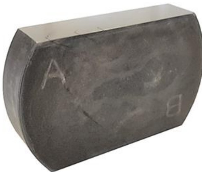
Fig. 1. The sample of 100Cr6 steel after quenching
