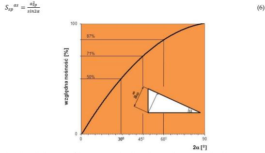
Fig. 7. The relative load capacity of the asymmetrical weld in relation to the symmetrical weld
