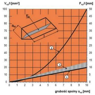
**Fig. 5.** Difference of strength increase (1) and volume (2) of symmetrical fillet weld with flat surface (3) – the area of possible increase in strength due to the increased penetration allowed by the standard EN 1993-1-8:2006
