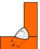
Fig. 3. Thickness of fillet weld a with deep penetration
