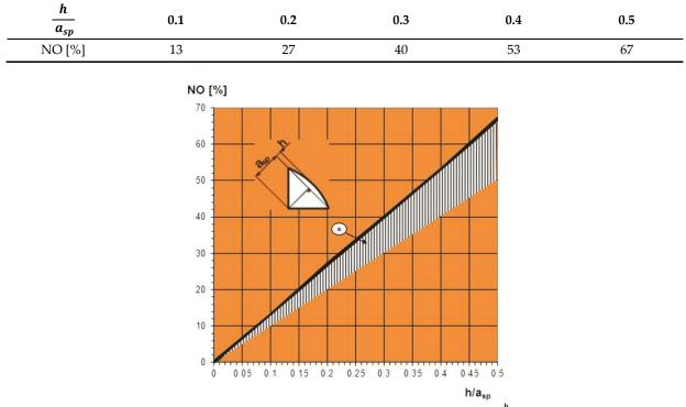
**Table I.** Useless volume (NO) of fillet weld depending on the ratio  $\frac{n}{a}$
