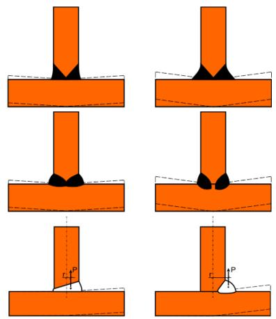
**Fig. 4.** Illustration of the formation of angular distortion in T-joints connected with various types of welds (P – force causing joint deformation, r – arm of force P between the neutral axis and the mass centre of the weld cross-section)
