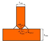
Fig. 1. Effective full penetration in T-joint with butt weld acc. EN 1993-1-8:2006
